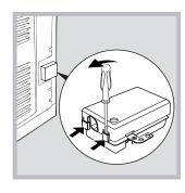
1. Open the terminal board by inserting a screwdriver into the side tabs of the cover. Use the screwdriver as a lever by pushing it down to open the cover (see diagram)
